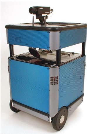
Figure 3: Pygmalion , the robot which was used in the experiments. It is a VME based system carrying currently a PowerPC card at 300 MHz. Besides wheel encoders and bumpers, the sensory system includes a 360° laser range finder and a gray-level CCD camera discussed in the second chapter. During the experiments it ran in a fully autonomous mode.
