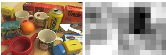
Fig. 2. Example of searching for the yellow soda can, placed closed to the center of the image. Dark areas indicate high likelihood of the object being present. There is a strong response where the soda can is placed, but also a small response at the location of the raisin box, standing to the left in the image, because of the similar yellow color.
