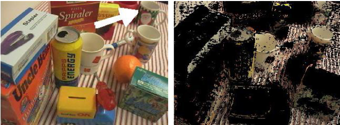
Fig. 1. Example when searching for the Santa-cup, visible in the top right corner. Left: The original image. Right: Pixels that survive the cluster assignment. The pixels that lie too far away from their nearest cluster are ignored (set to black in this example). The red striped table cloth still remains, as the Santa cup contains red-white edges.
