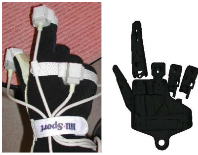
Fig. 9. An example mapping of a human pointing grasp using the Robonaut Hand.
