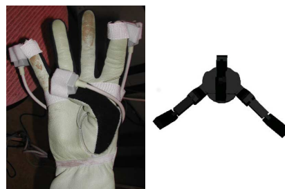
Fig. 7. An example mapping of a human grasp using the Barrett Hand.
