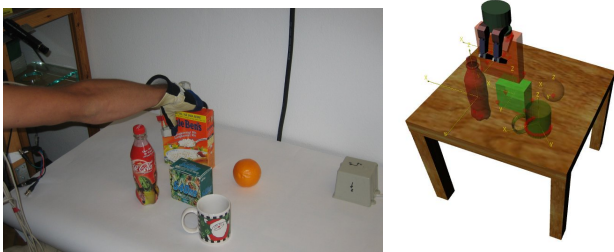
Fig. 3. Left: The human moves the rice box. The system recognizes what object has been moved and which grasp is used. Right: The robot grasps the same object using the mapped version of the recognized grasp.
