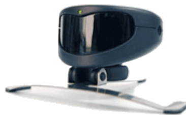
Figure 4. The TrackIR head tracker.
