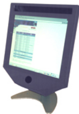
Figure 2. Tobii Technology ET-17.
