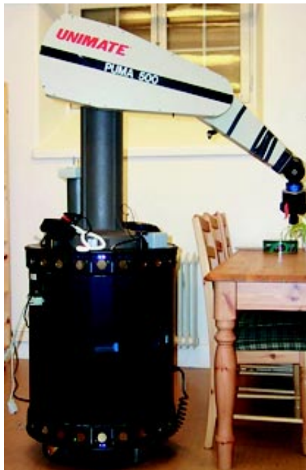
The Nomad XR4000 with the onboard Puma 560
